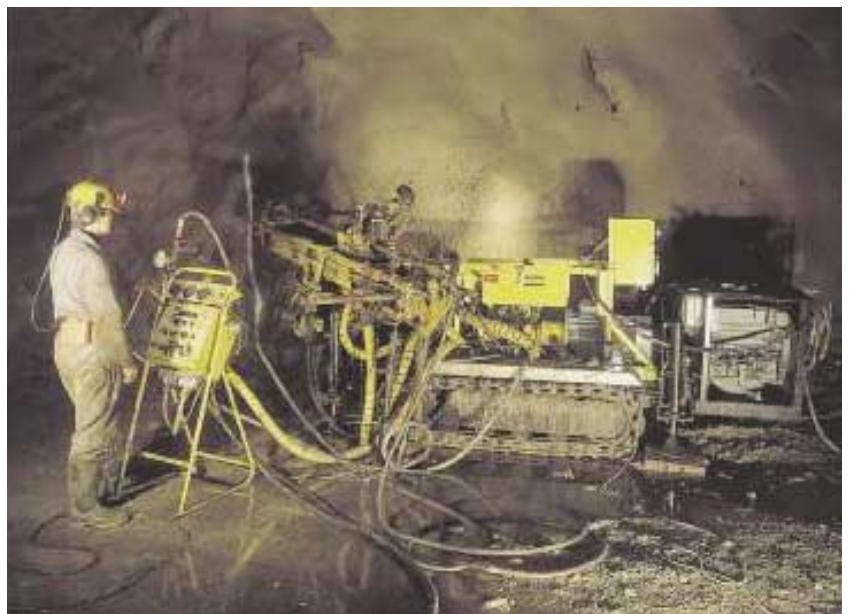
Atlas Copco Craelius Diamec 264 APC at work underground.
