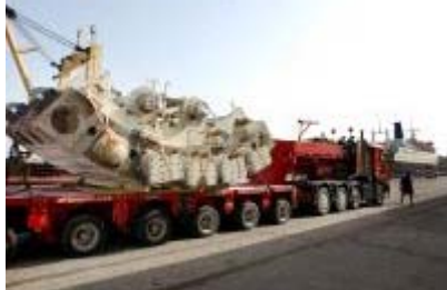
Picture 1: Pieces of the Robbins/Mitsubishi TBMs loaded onto lorries in Malaga harbour.
