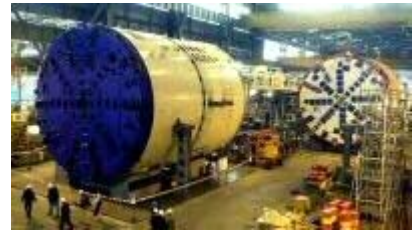
Picture 1: The two TBMs for the Abdalajís tunnels on the Córdoba-Málaga high speed line.
